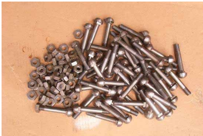
New hub nuts and bolts – Unfortunately these cannot be bought in this size so new ones were made from scratch.
