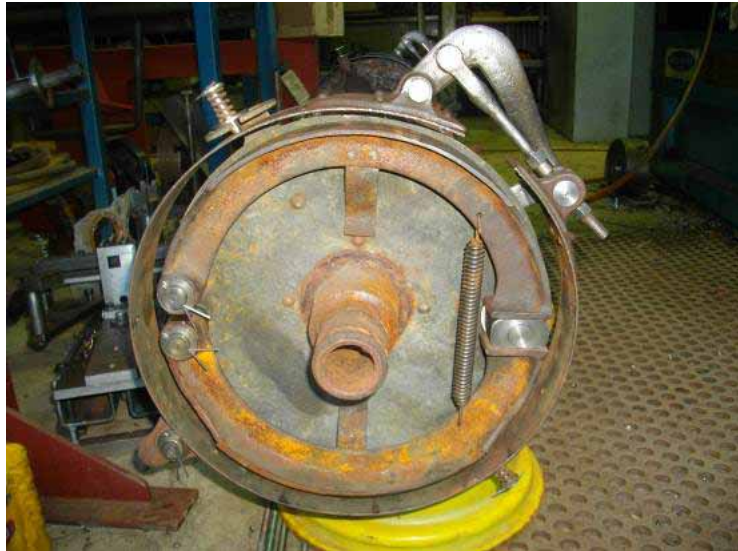
Brake shoes and external brake bands (note new brake cam and pins).
