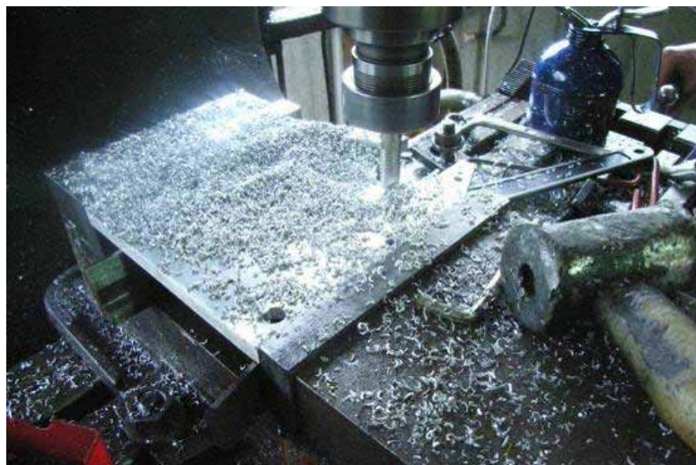
Machining the back out of the gear change side cover plate.
