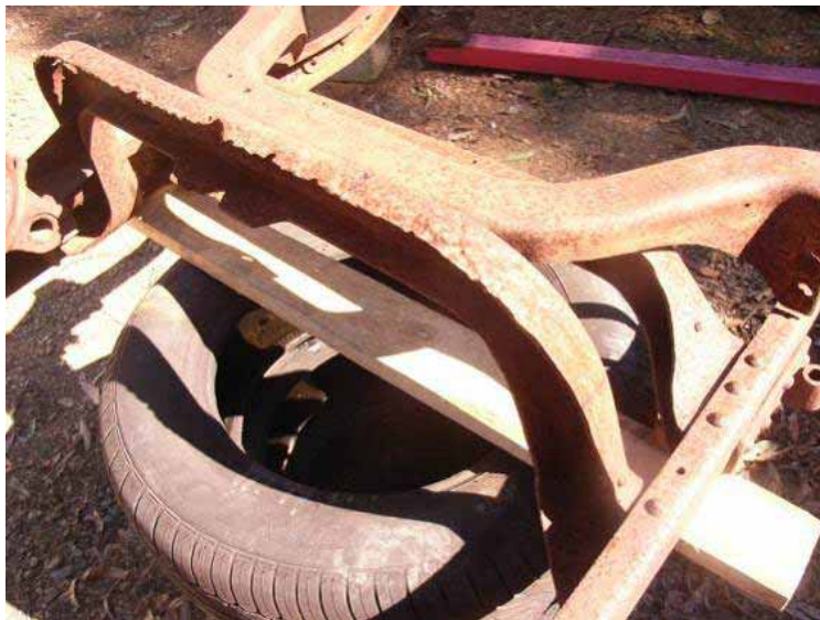
Rust damaged front cross member needing replacement.
