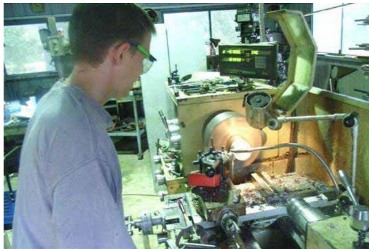
Doing some turning on the lathe for ignition and throttle control gear blanks.
