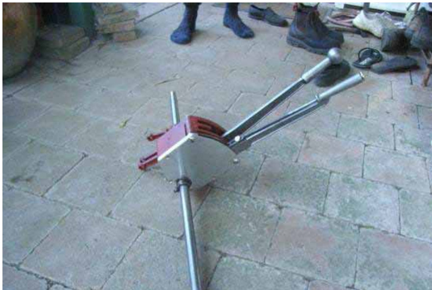
Rebuilt gear change and hand brake mechanism with new aluminium side plate.
