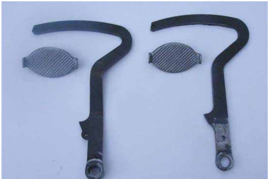
Laser cut clutch and brake pedals along with pedal pad castings. I redrew the factory drawings of these in AutoCAD and had them laser cut from 10mm mild steel plate.
