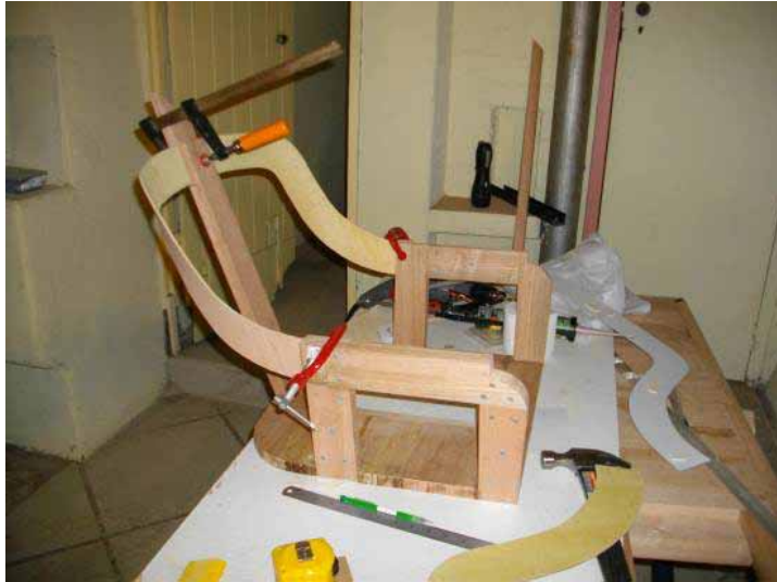
First layer of plywood in position for lamination of the back of the seats.
