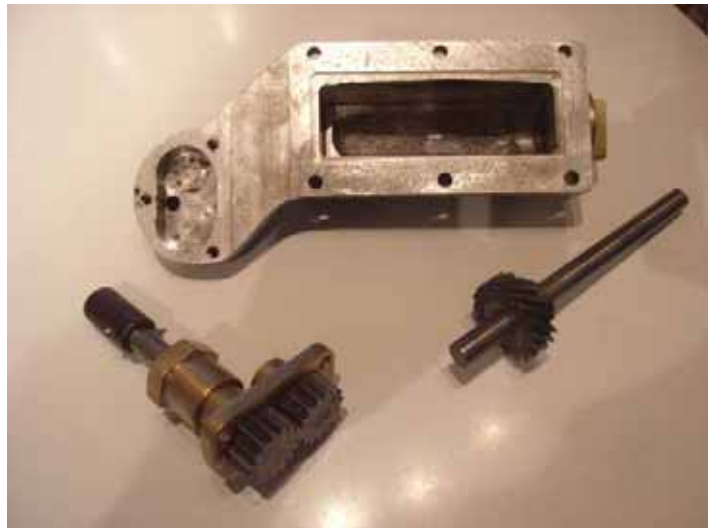
Oil pump casting after machining with oil pump mechanism.
