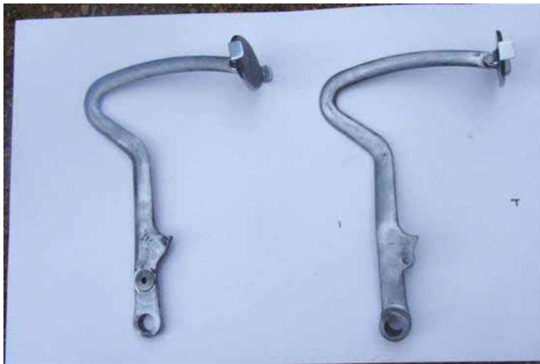
Aforementioned pedals after being finished and shaped with angle grinder. These pedals are particularly special as their shape is specific to the speedster model, making originals almost impossible to find.
