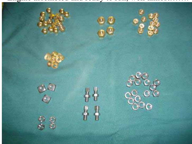
New hand made nuts and bolts for engine – all made as copies of originals to get the right hex sizes.
