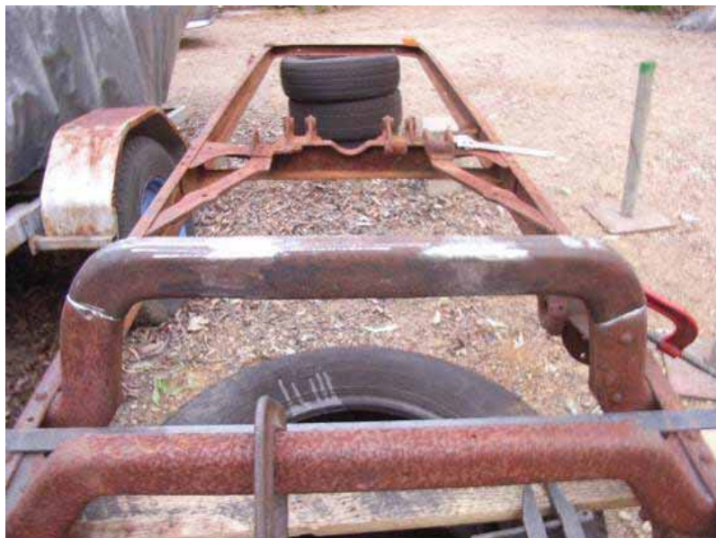
New front cross member fabricated from bits of old chassis's tacked in place
