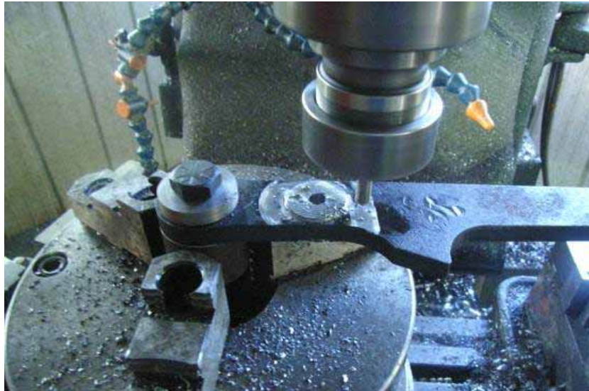
Machining the special radial grooves for the clutch pedal adjustment.
