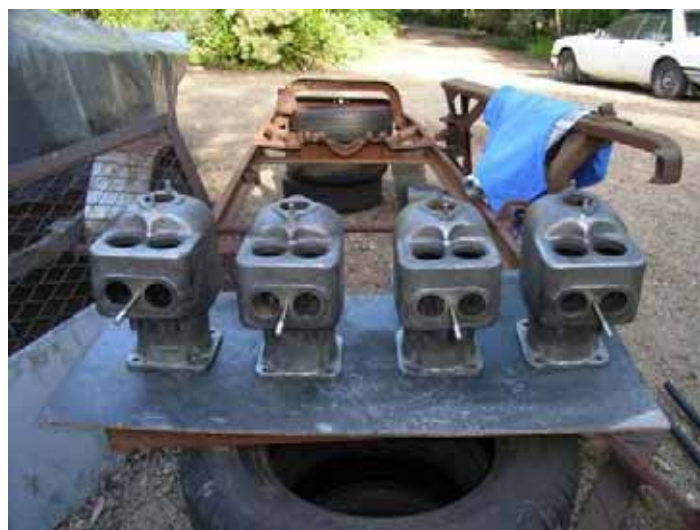
Cylinder pots taken off, cleaned up and new manifold studs installed.
