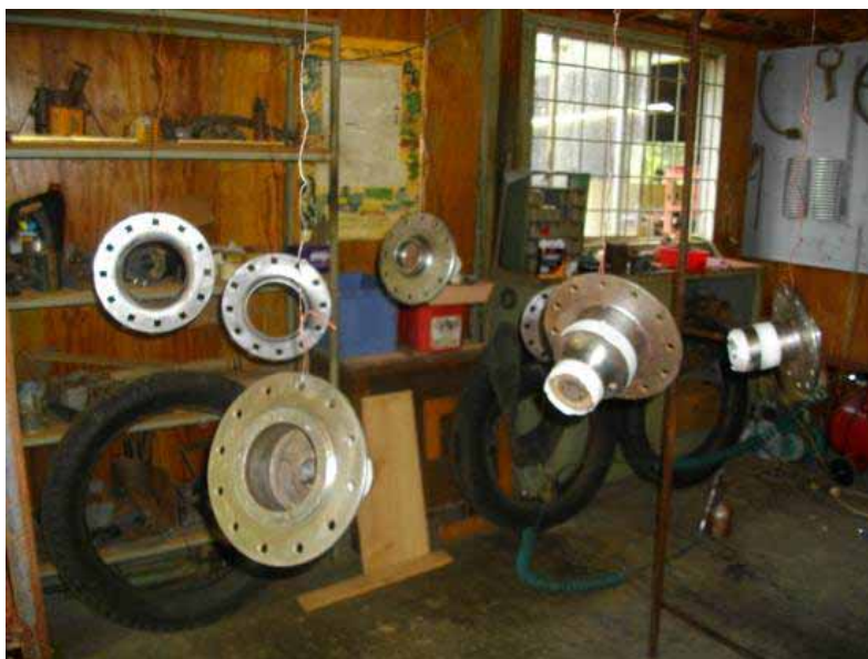
Hubs rebuilt and cleaned up ready for painting.
