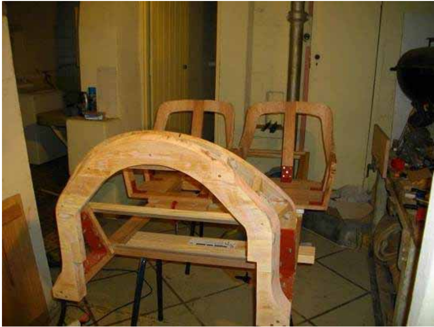
All the woodwork for the body I have done myself, under my flat in Brisbane. The overall dimensions are as per factory blueprints.
