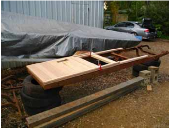
Start of the body, checking to make sure the base fits the chassis.
