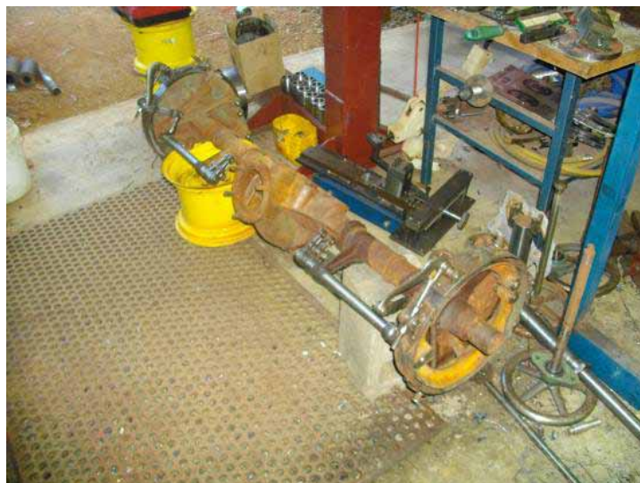
Back axle with rebuilt brake mechanisms.
