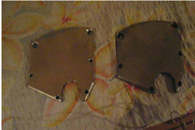
New gear change side cover plate on the left, a borrowed original one that was copied on the right.
