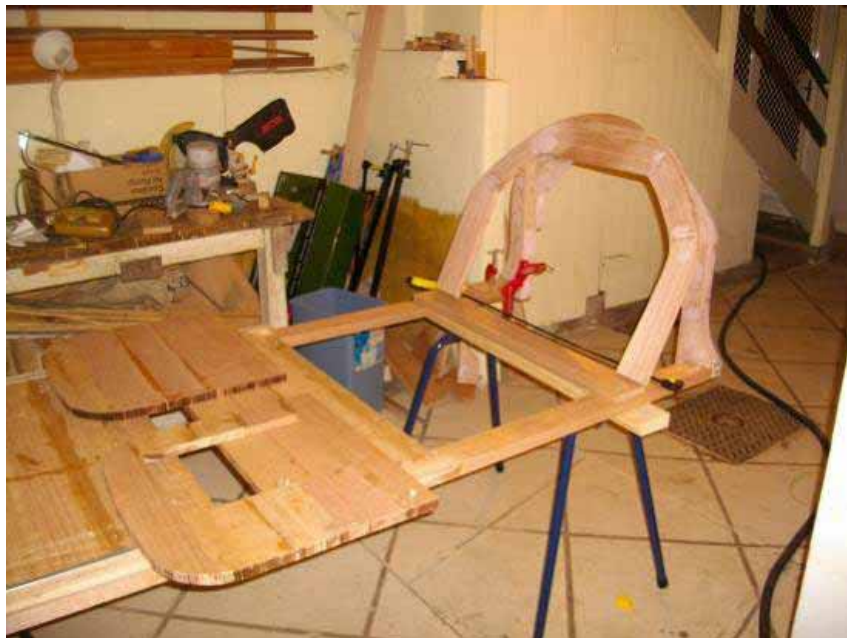
Bodywork progressing: Trial assembly of dash and cowl with seat bases.
