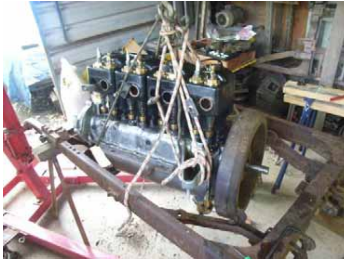
Engine now re-assembled being lowered into the unused chassis.
