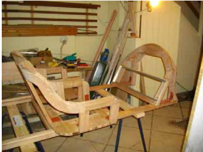
Body frame almost finished and ready for panelling.
